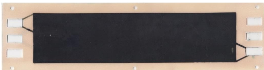
Figure 3. Image of the membrane MK-40 modified by polyaniline (active area 5 \times 20 \text{ cm}^2 ).
