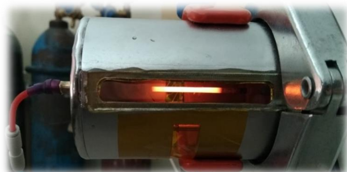
Figure 1. Direct AC/DC heating of hollow fiber membranes.
