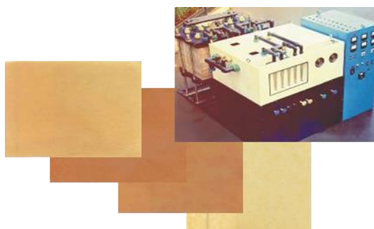
Figure. Electro dialysis unit EDA 1 - 400 × 60 and samples of synthesized anion- and cation-exchange membranes for water purification.
